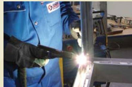
Net fasteners are inserted into the goal frames first and then welded!
